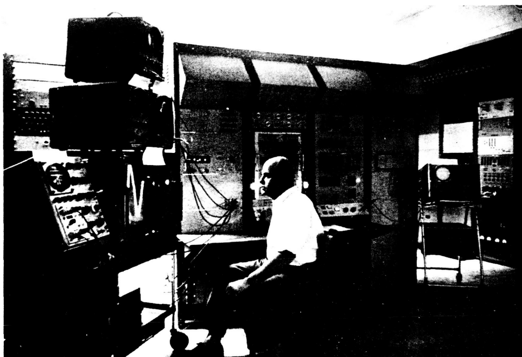
Fig. 4. Operating with signal frequencies as large as 60 kHz, the digitally controlled ASTRAC II here displays the complete input-output cross-correlation function of a fast-time simulated control system with
