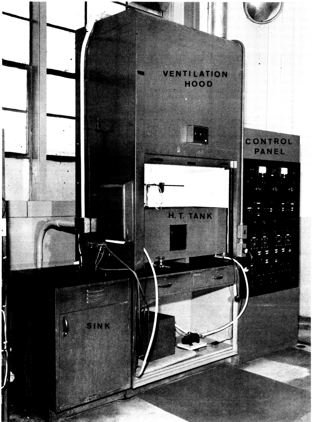
FIGURE IV-3 This Photograph Shows the Heat Treat Area of the System Which Includes the Control Panel, Heat Treat Tank, Ventilation Hood, and Sink
