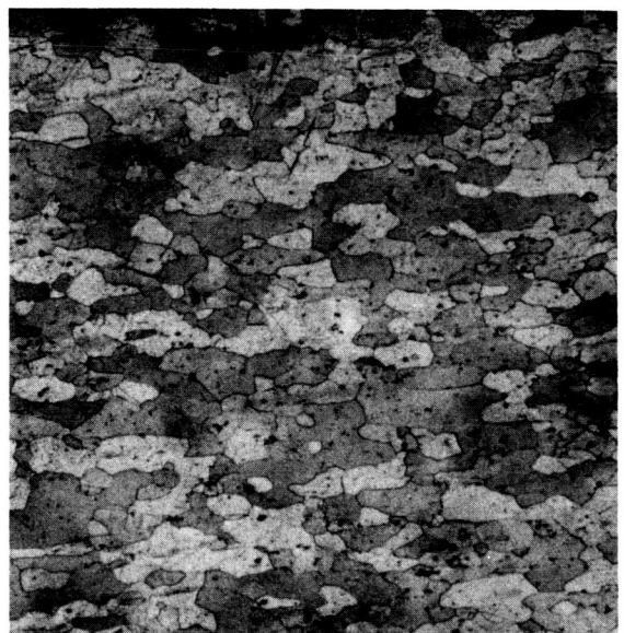
MAG: 100X Figure V-22 Etch: Kellers General structure of a 2219 Al specimen electrolytically solution treated at 1000°F for 60 seconds and quenched.
