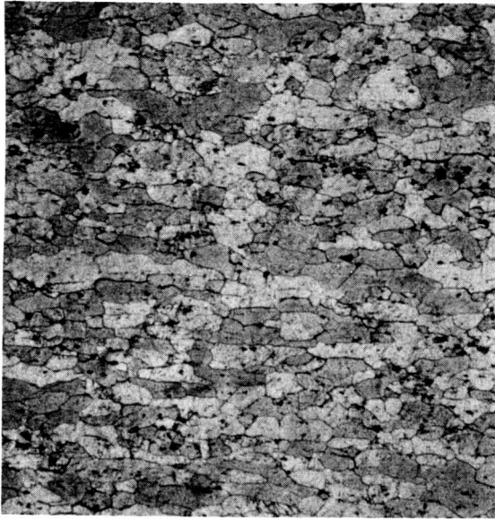
MAG:100X Figure V-19 Etch:Kellers General structure of a 2219 Al specimen, conventionally solution treated at 1000°F for 45 minutes and water quenched.
