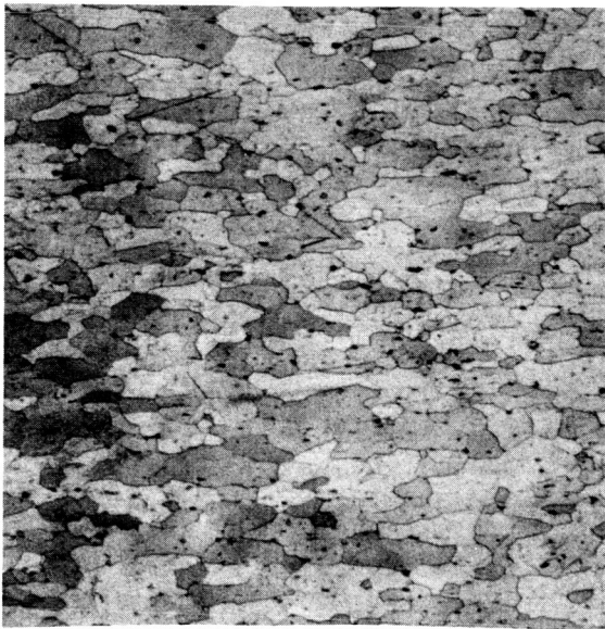
MAG: 100X Figure V-21 Etch: Kellers General structure of a 2219 Al specimen electrolytically solution treated at 1000°F for 45 seconds and quenched.
