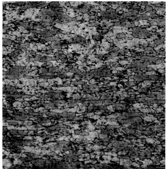
MAG: Figure V-20 Etch: Kellers General structure of a 2219 Al specimen electrolytically solution treated at 100°F for 30 seconds and quenched.
