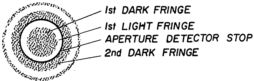
Fig. 5 Interferometer Fringe Field For v_{\max} and L_{\max}
