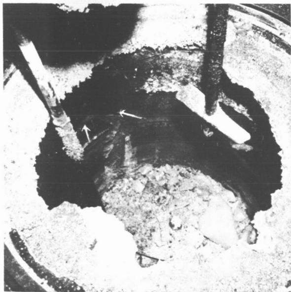
Interior of Cell Showing Damage of Glass Liner, Protective Glass Tubing Around Stirrer Shafts Lost. (White Lump in Cell is Dry Ice).
