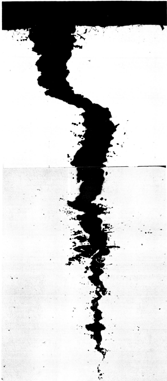
Fig. # 8 Metallographical Crossection of Failed Ring - Note Crack Propagates Through Defect Area
