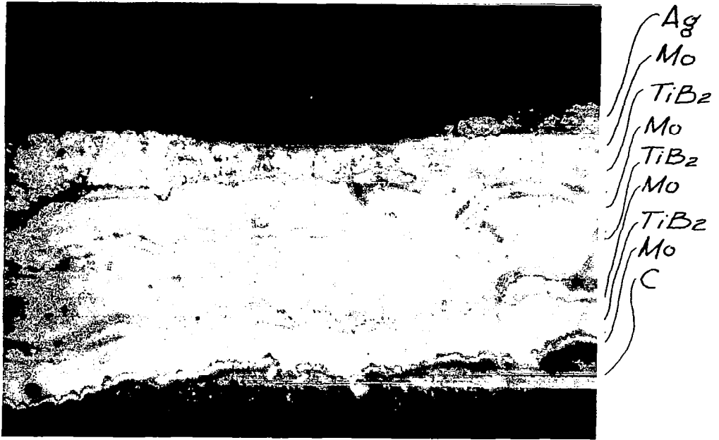
Figure 60. A Seven Layer Mo-TiB 2 Composite
