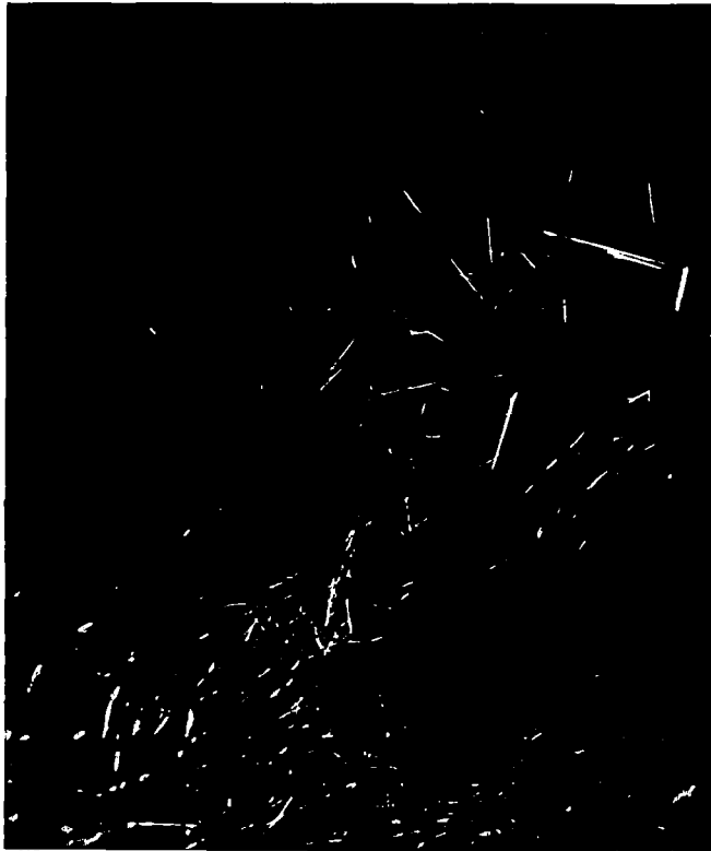
Figure 65. Texture of as Grown SiC Whisker Wool
