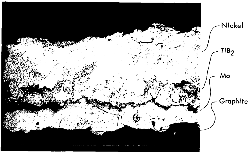
Figure 59. Mo and TiB 2 Vapor Deposited onto a Graphite Substrate 200X
