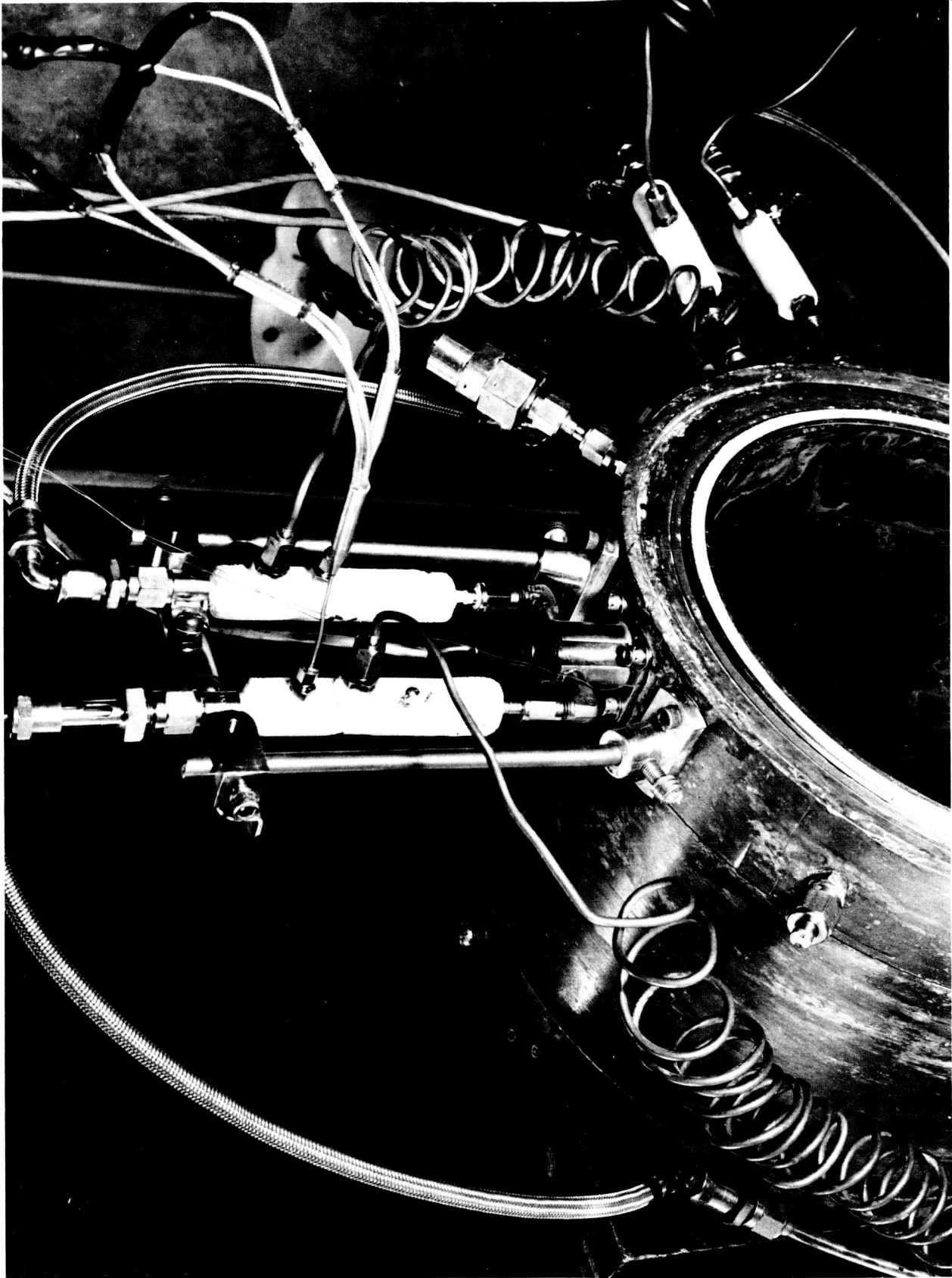
Photograph of Two Dynisco Model PT49CF Transducers Installed in a Research Rocket Thrust Chamber
