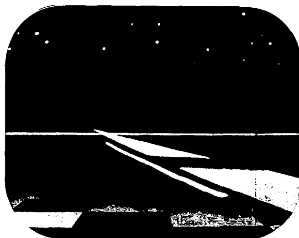
VEHICLE AT REQUIRED ALTITUDE BUT TO LEFT OF NOMINAL PATH. ON INTERCEPT COURSE.
