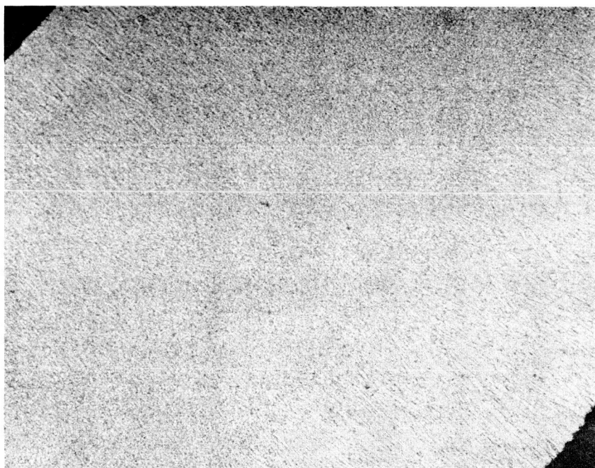
Fig. 7--Vapor-deposited tungsten containing an average of (a) 262 ppm and (b) 270 ppm. Carbon added during deposition from \text{CH}_4 : \text{WF}_6 : \text{H}_2 volume rates of 1.4:1:3.1 and 2.6:1:2.7, respectively
