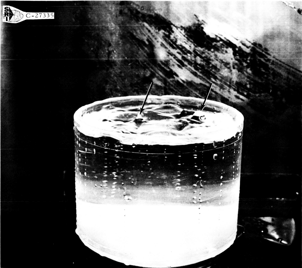
Figure 14. Photograph Of Unstable 1/2 Subharmonic Large Amplitude Response
