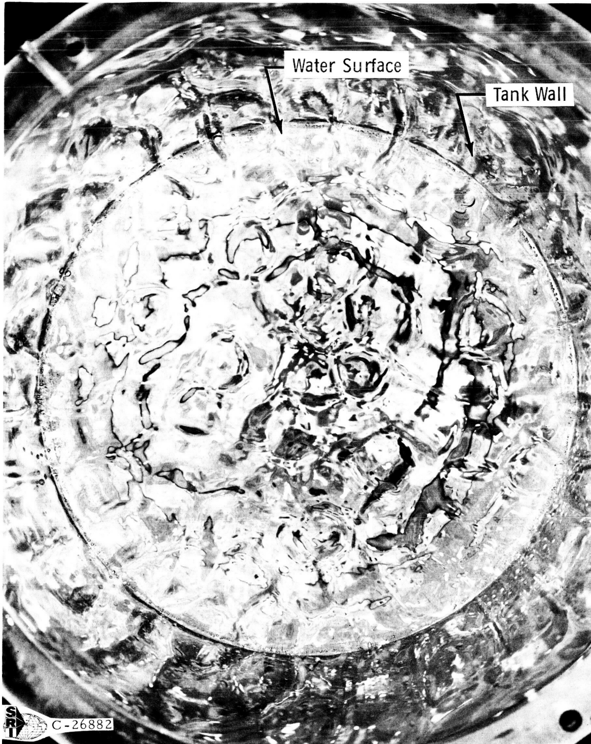
Figure 7. Overhead Photograph Showing 1/2 Subharmonic Response With Equal Distribution Of Wavelets
