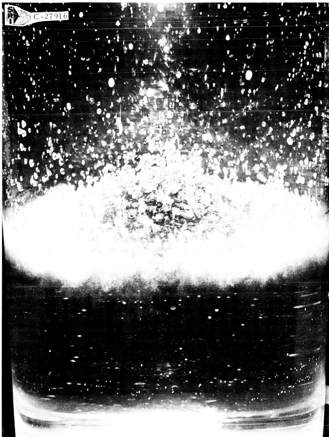
Figure 3. Spray Excited First Symmetric Mode In A 24.8-cm Cylindrical Container
