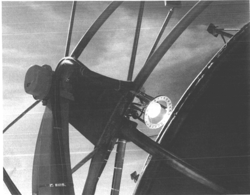
Fig. 17. Calorimeter test focal-zone setup, open, operating
