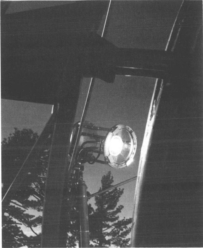
Fig. 16. Calorimeter test focal-zone setup, windowed, operating
