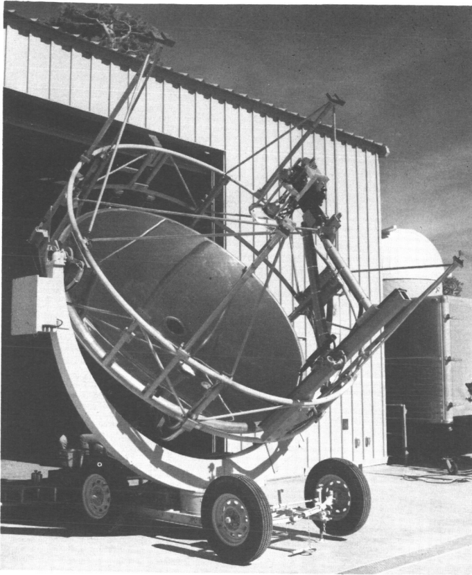
Fig. 14. Calorimeter test in operation
