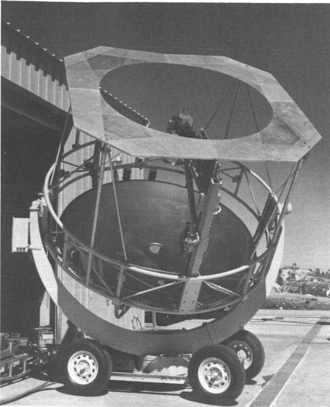
Fig. 18. 7.5-ft-diam. -opening mirror-mask calorimeter test in operation
