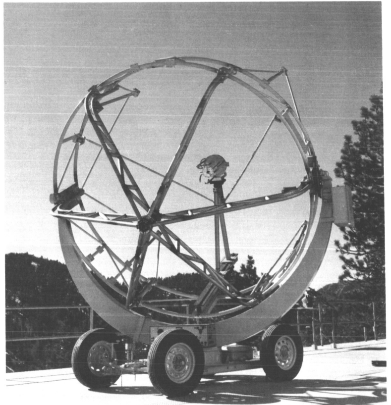
Fig. 2. Solar tracker structure prior to installation of 9.5-ft-diam. concentrator S/N 1
