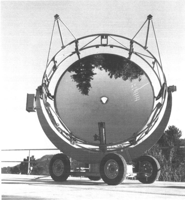
Fig. 1. 9.5-ft-diam., 45-deg-rim-angle electroformed solar concentrator S/N 1 during installation
