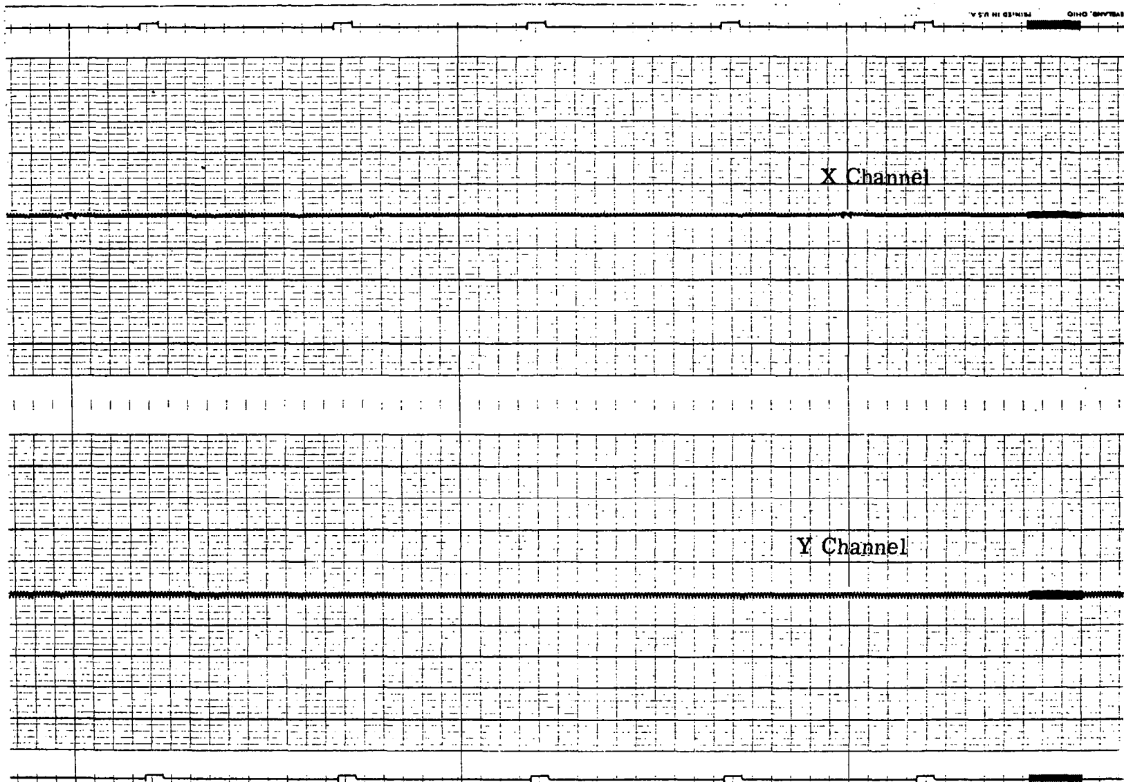
Figure 4.7 PUPIL INTEGRATOR OUTPUT WITH OCULOMETER IN RESET MODE (All loops open) -- 20 mv/line
