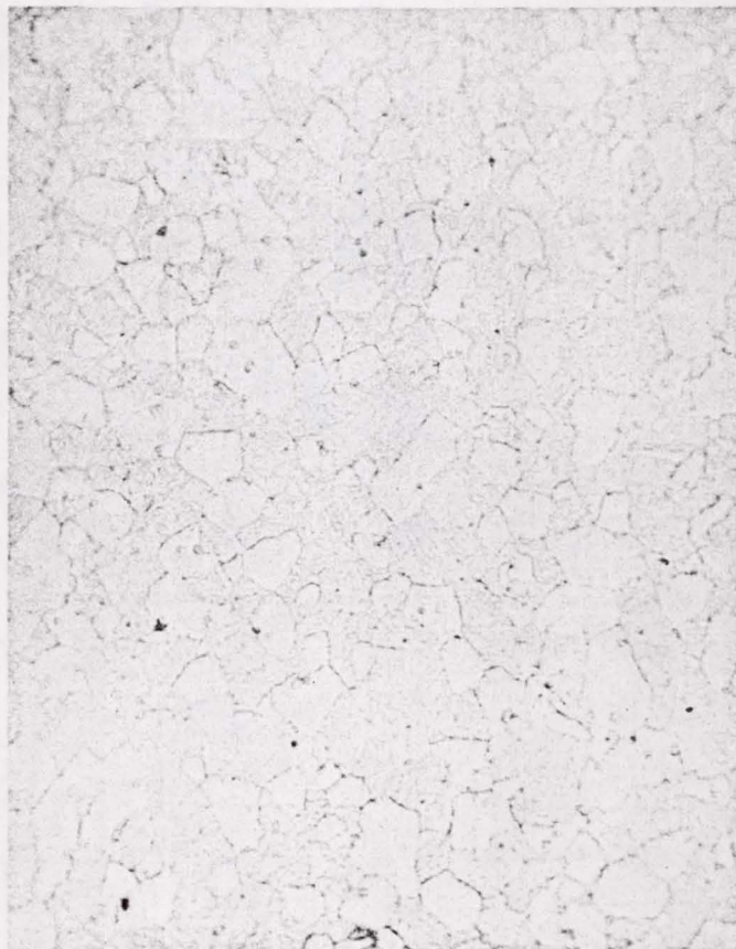
Figure 1-4. Tufftrided Gear from the Second Set Processed Showing Approximately 30% Ferrite (500x)
