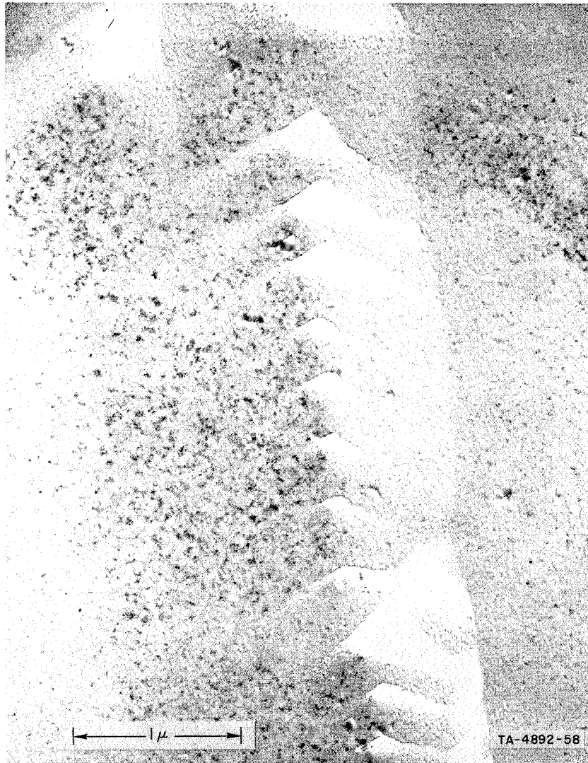
FIG. 18 DISLOCATION ETCH PITS IN TaC 0.9 SUBGRAIN BOUNDARY
