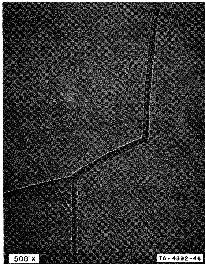
FIG. 19 SUBGRAIN BOUNDARIES IN SINGLE CRYSTAL OF HAFNIUM CARBIDE (1500X)
