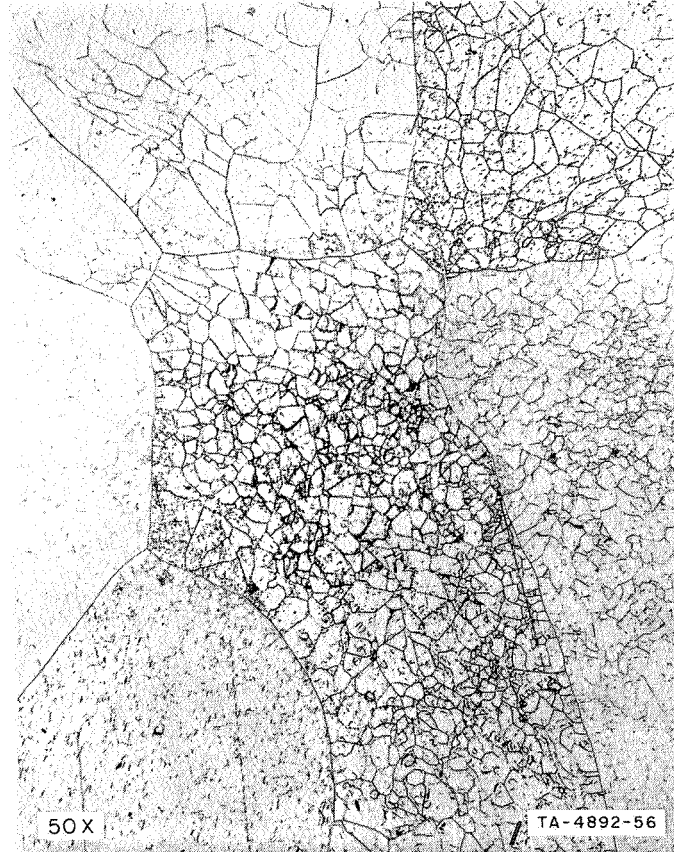
FIG. 16 ETCHED TaC 0.9 WITH GRAIN BOUNDARIES AND SUBGRAIN BOUNDARIES (50X)
