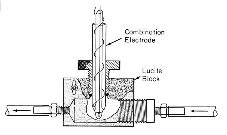
Figure 4 - Density control (sample) chamber, actual size.
