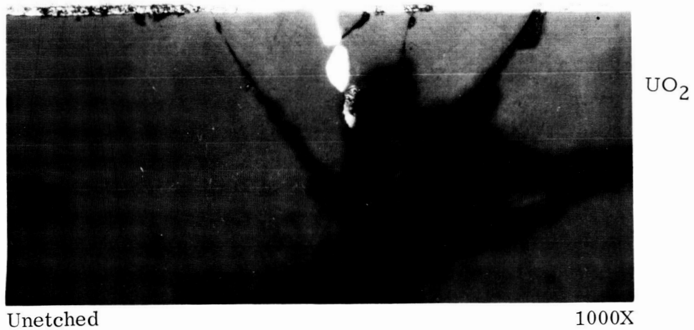
FIGURE 14. THIN LAYER OF METALLIC APPEARING PHASE ALONG THE INTERFACE BETWEEN UO 2 AND END CAP CAPSULE 11 (2200°C - 500 hours) 2
