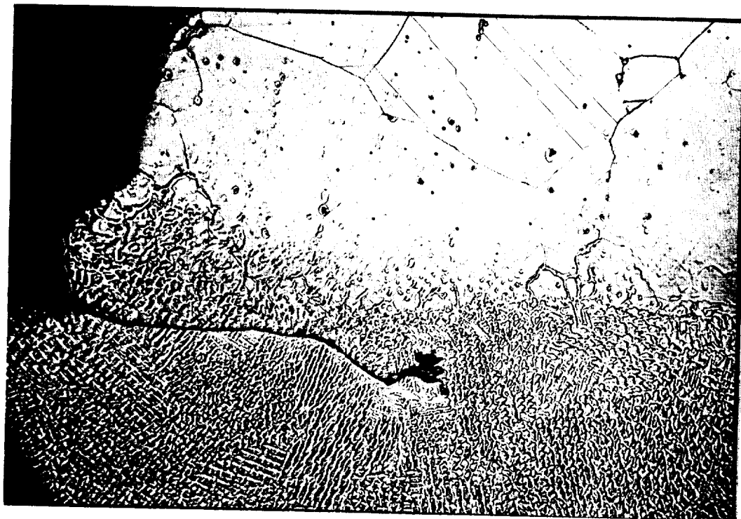
FIGURE 5 - Microstructure of welded end cap section 7-1 in as-formed condition.
