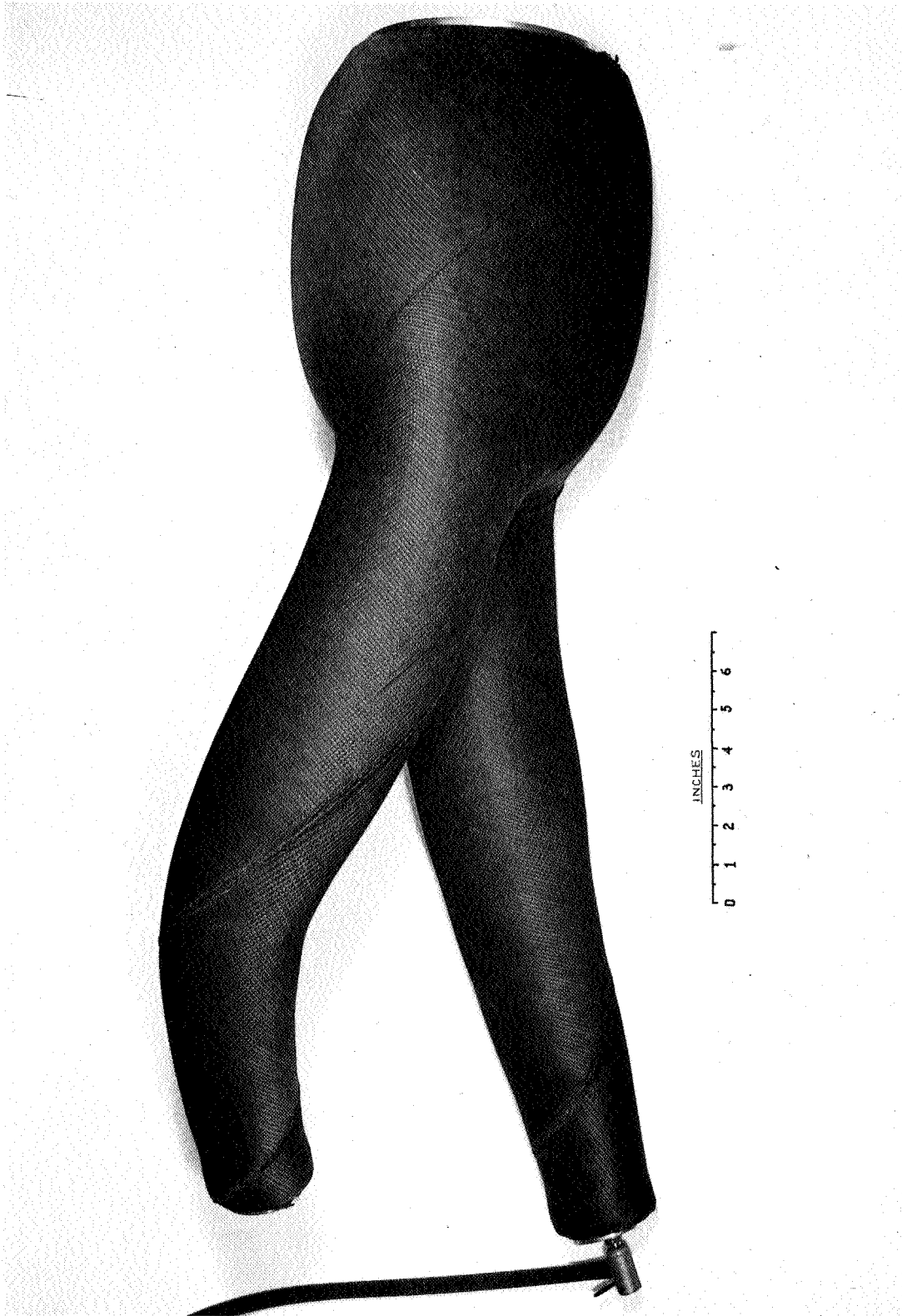
FIGURE 14. DEFORMATION OF BIFURCATED SLIP-NET STRUCTURE - 7 PSI INTERNAL PRESSURE
