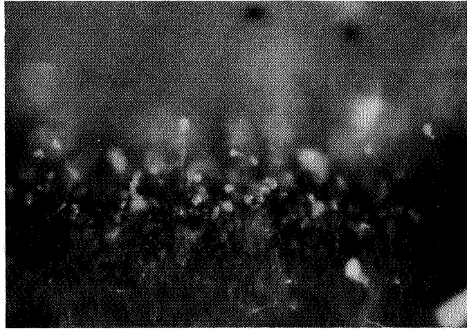
140X Photomicrograph of Whisker Growth on Vapor Transport Film
