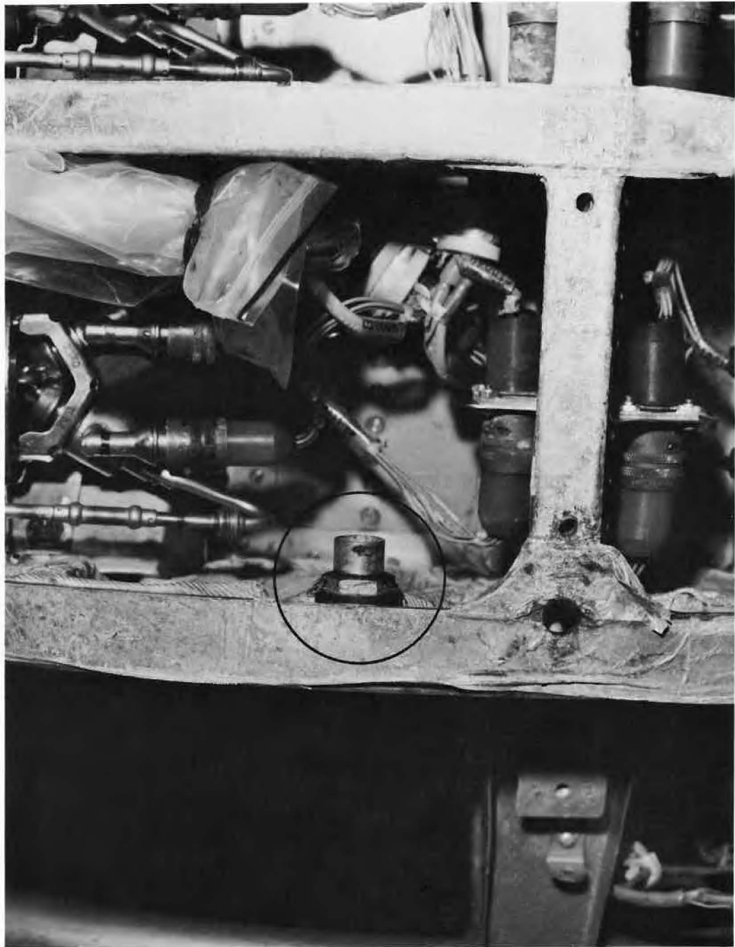
Figure 12-10 - Sheared connector to R and R separation igniter.
