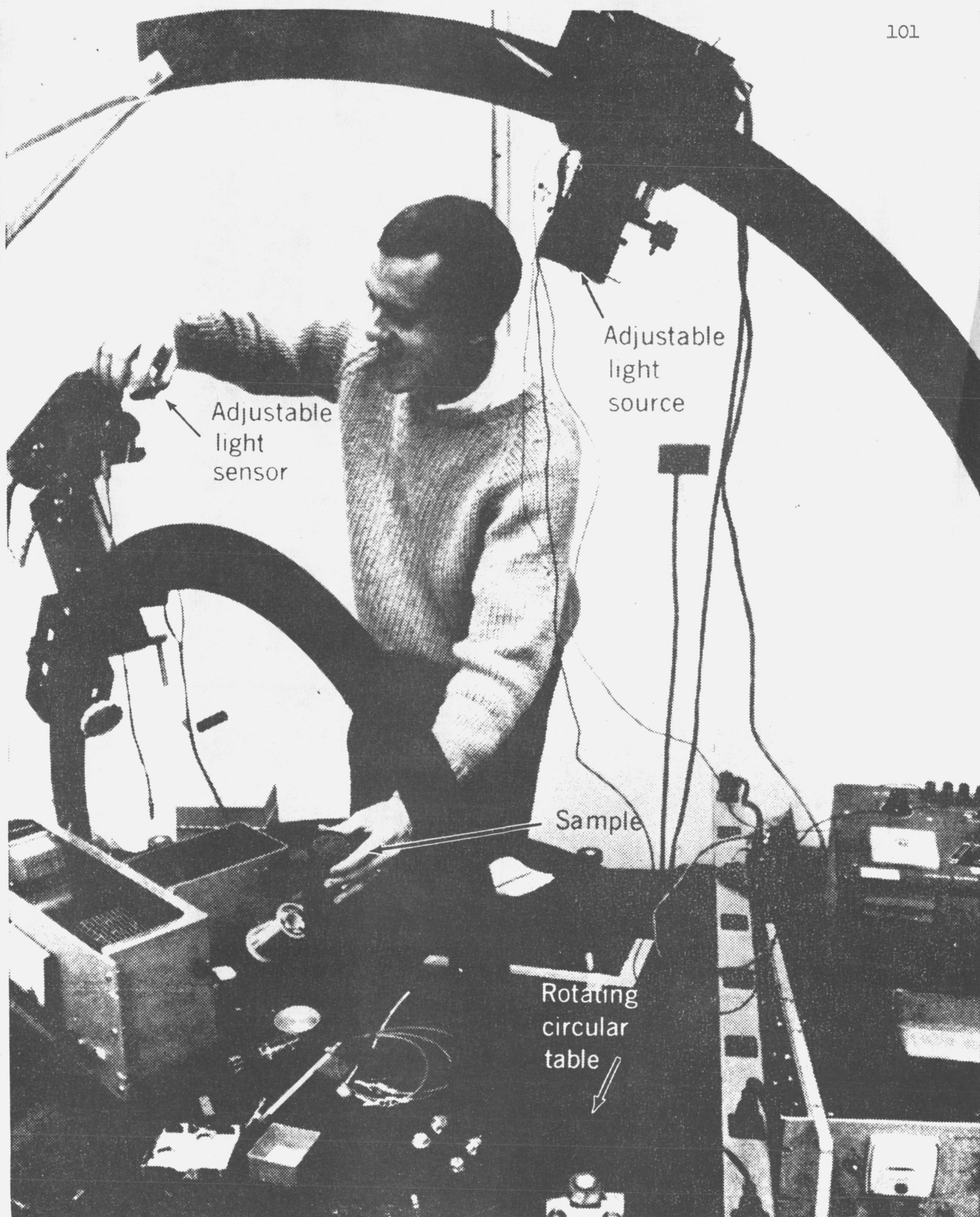
Fig. 27. Photograph of author operating the reflectometer-polarimeter (from the March 27, 1967, issue of Product Engineering).
