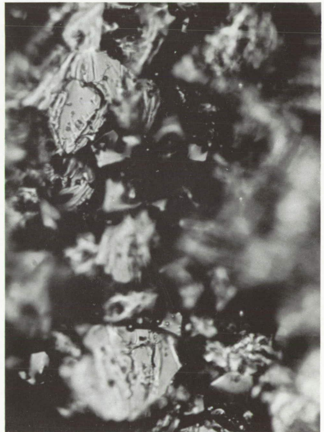
Fig. 5. Fracture surface of TaC run 48 showing planar grain surfaces
