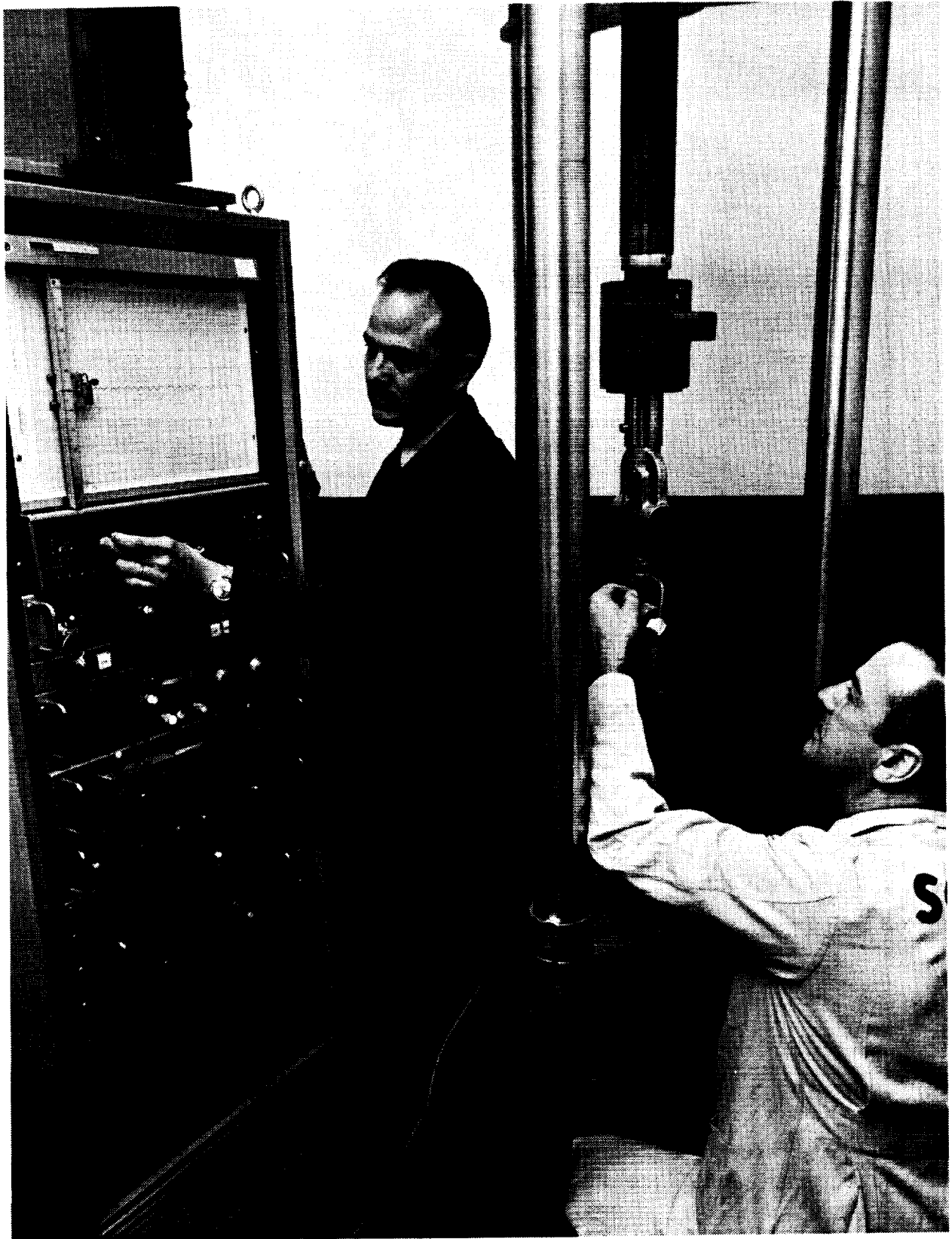
FIGURE 5. MTS AXIAL FATIGUE CLOSED LOOP TESTING MACHINE
