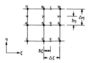
Figure 3.2 - Showing a 3 x 3 grid of points and intermediate points on one grid line only.
