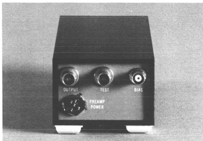
ND-525HRP High Resolution Preamplifier rear panel showing Output, Test, Bias, and Preamp Power connectors.
