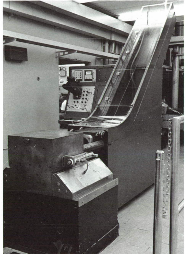
Fig. 6. Inclined ramp impact testing device
