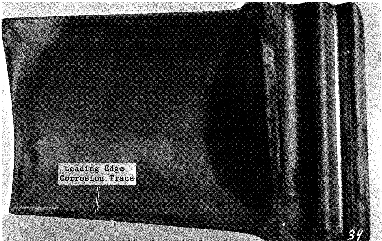
Figure 55. Concave Side of U-700 Second Stage Turbine Blade After 2000-Hour Endurance Test. (C66011345) Mag: 5X
