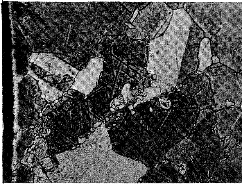
Figure 6. First Stage U-700 Blade Dovetail After 2000-Hour Endurance Test Showing Concentration of Accicular Structure Presumed to be Sigma Phase. (B322411)
