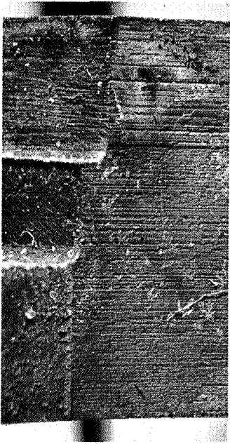
Figure 89. Liquid Potassium Impact Surface of Recrystallized TZM Erosion Insert Specimen Number B-2. Mag: 9X (C66012761)
