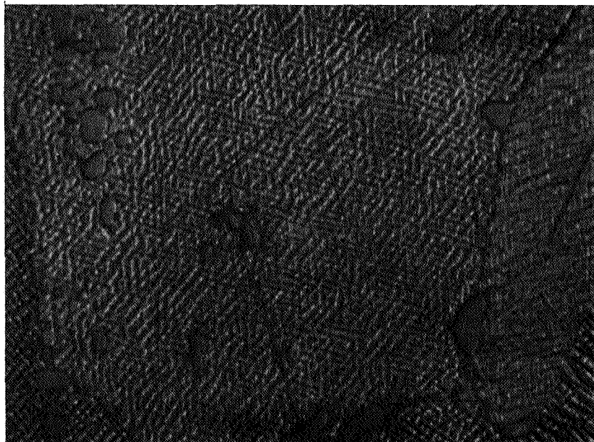
Figure 7. First Stage U-700 Blade Dovetail After 2000-Hour Endurance Test Showing Concentration of Accicular Structure Presumed to be Sigma Phase. (B322311)
