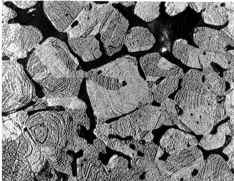
Figure 102. Cross Section of Metallic Deposit from CD Nozzle Test, 100X (Top); Enlarged and Etched Section of Metallic Deposit from CD Nozzle Test Showing Vapor Deposition Characteristics, 1000X (Bottom). (C63121252)
