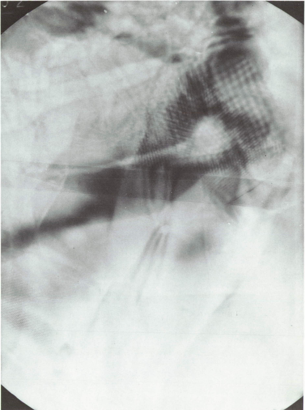
Fig. A-3. Transmission electron photomicrograph of deformed pyrolytic carbon (20,000 X)
