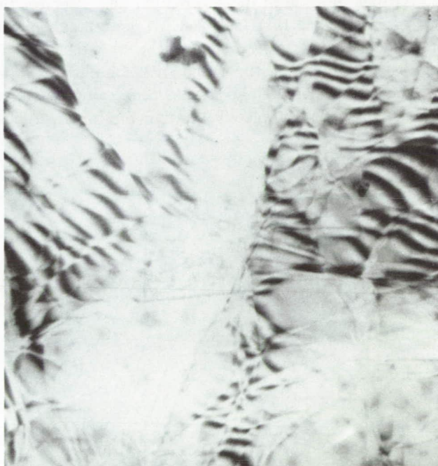
Fig. 7. Typical dislocation pattern in hot-worked graphite: transmission electron microscopy (10,000 X)
