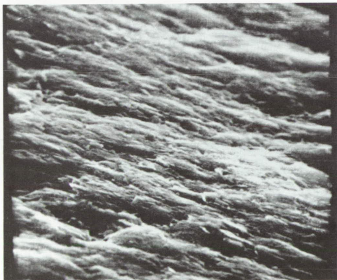
Fig. 5. Unpolished side view of 27%-deformed specimen, by scanning electron microscopy (3,500 X)
