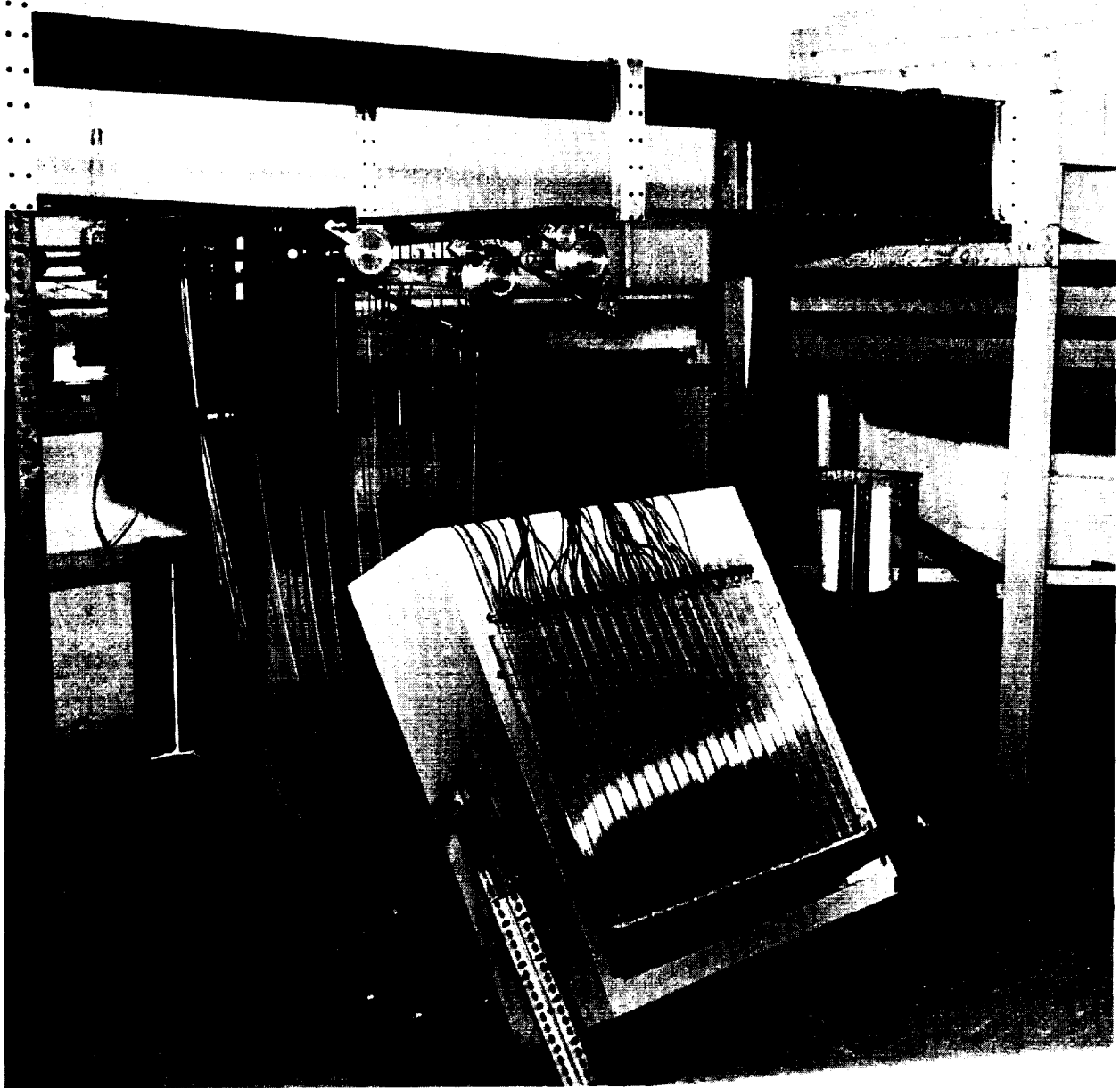
Figure 1. View of Working Section of Wind Tunnel, Showing Bell Mouth Intake, Multitube Manometer and Adjustable Separated Flow Working Section Installed.
