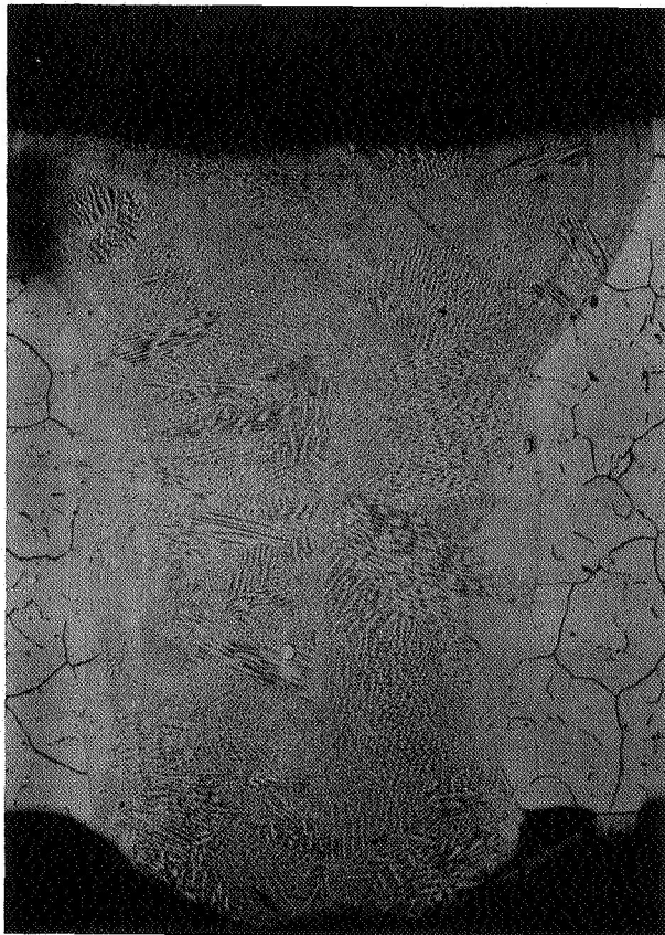
(3) Electron beam weld: sound, fine grained weld with fine precipitate. 50X
