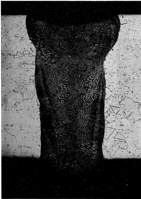
(3) Electron beam weld: sound, no voids, very fine-grained cast structure. 50X
