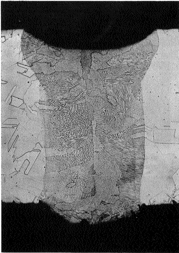
(3) Electron beam weld: sound weld, as-cast structure with very fine precipitate. 50X
