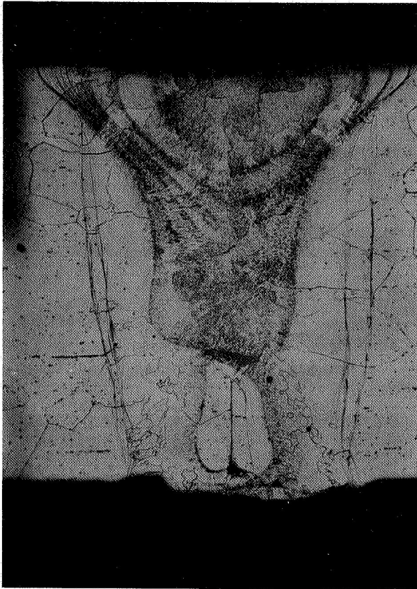
(3) Electron beam weld: very fine grain weld zone, some lack of fusion at bottom of weld. 50X
