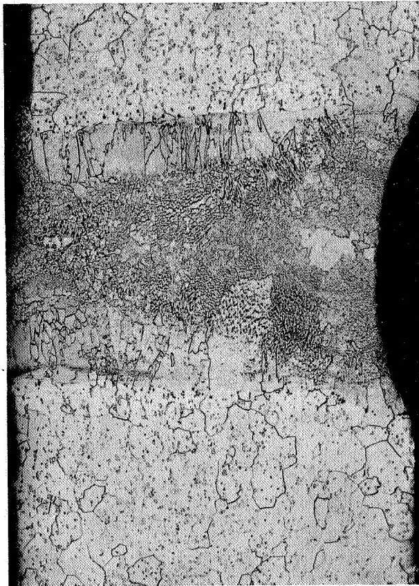
(3) Electron beam weld: sound, fine grained weld. 50X
