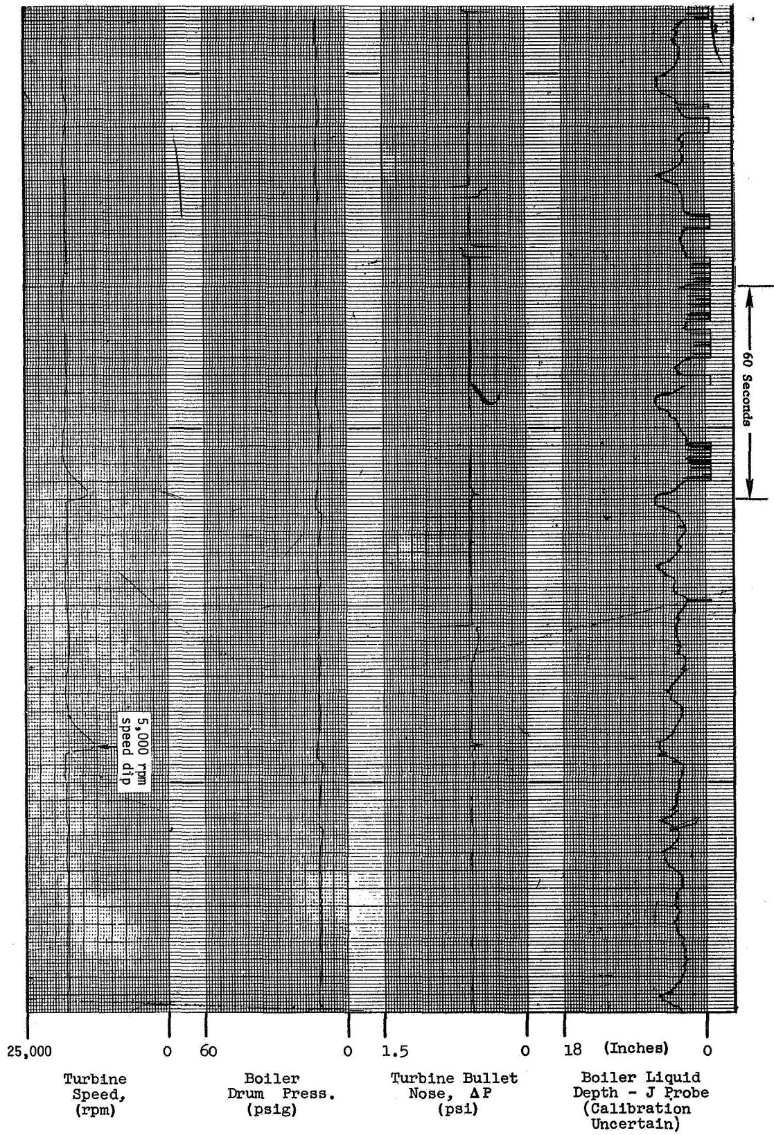
Figure 20. Boiler Liquid Level Gage, J-Probe.
