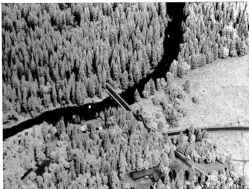
Infrared film and Wratten 89B filter; poor shadow penetration is one of the drawbacks in using this film-filter combination. The light tone with which vegetation registers makes this film-filter combination a good one to include in multiband photography that seeks to provide unique tone or color signatures for various objects and conditions.
