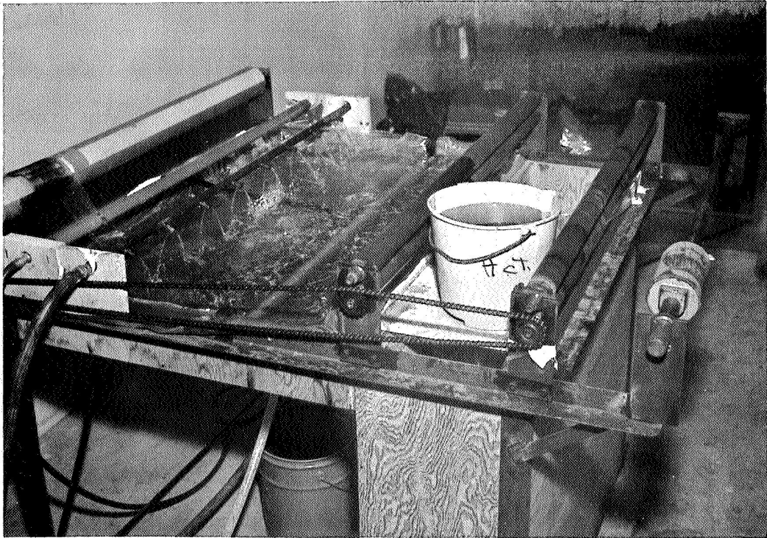
Figure 8 Single Tank Plating Equipment
