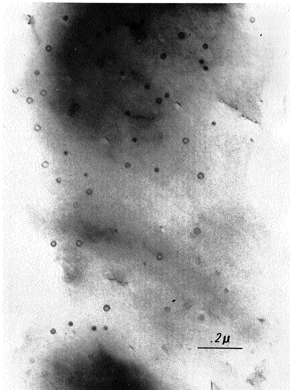
Figure 35.--Isolated colony of voids in a foil that was annealed for 100 hours at 500°C. Average void diameter is 300 Å.
