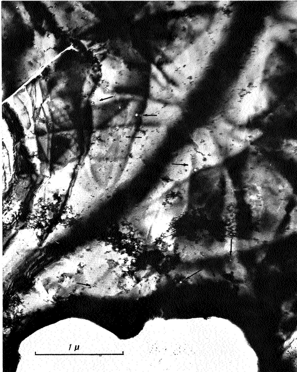
Figure 25.--Polyhedral voids in pulse quenched platinum foil after partial melting in the electron microscope. The average void size is approximately 300 Å.
