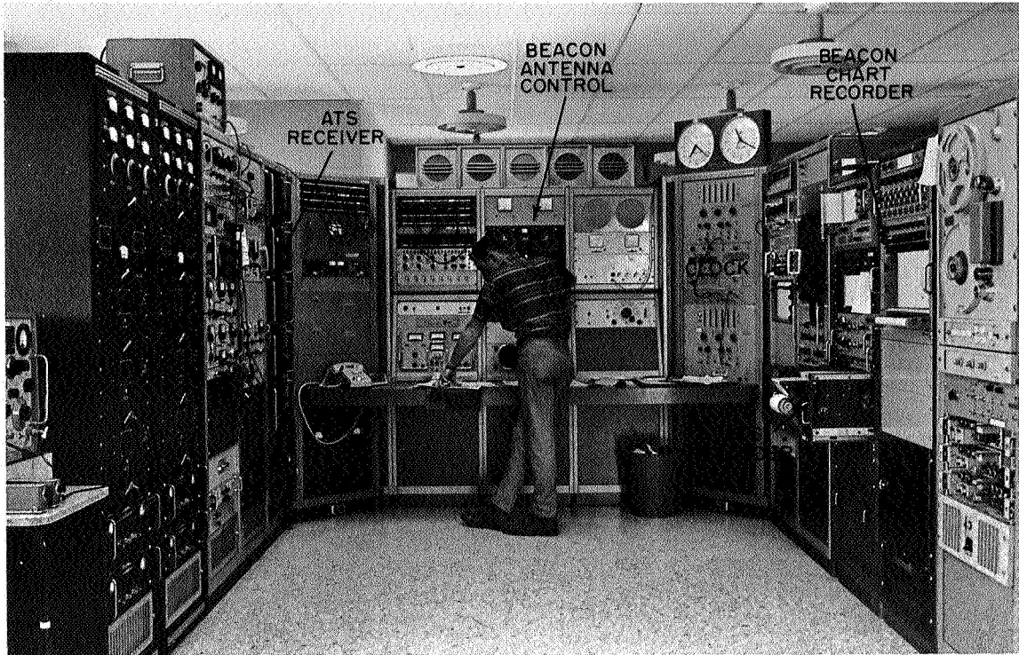
FIG. 4-18. THE BEACON SATELLITE TRACKING STATION AT STANFORD. The operator is reading azimuth and elevation from an ephemeris, and pointing the antenna. ATS receiver and chart recorder are also located here.
