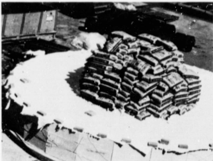
Fig. 17. Sandbags used to stress center of mirror
