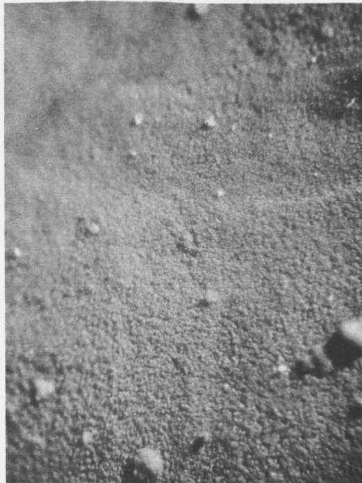
FIGURE 11. AlP DEPOSITED ON GaAs BY THE \text{AlCl}_3\text{-PH}_3 PROCESS
