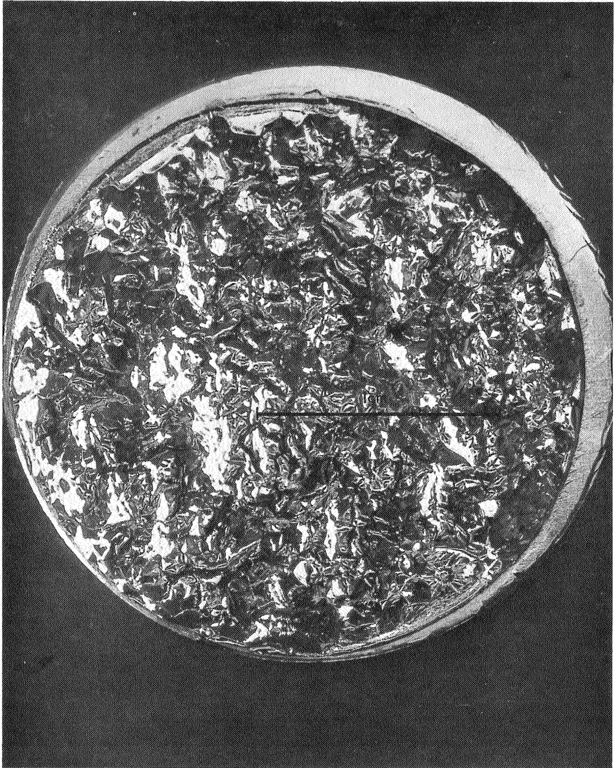
Figure 53: STRETCH-FORMED ALUMINUM MIRROR AFTER HEATING TO 200°C
