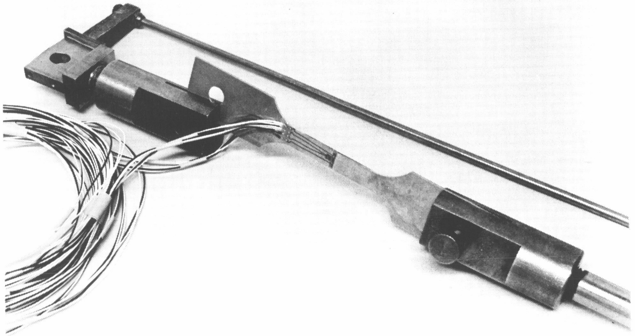
Figure 20. Strain Gaged Sheet Tensile Test Specimen in Quick-Release Clevis
