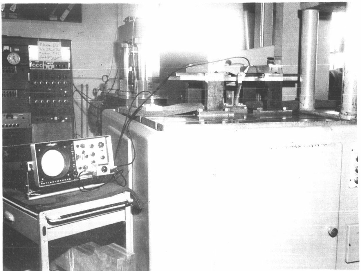
Figure I-5. Ultrasonic Test Instrumentation Used During Cyclic Flaw Enlargement on the One-Inch-Thick Plate Specimens
