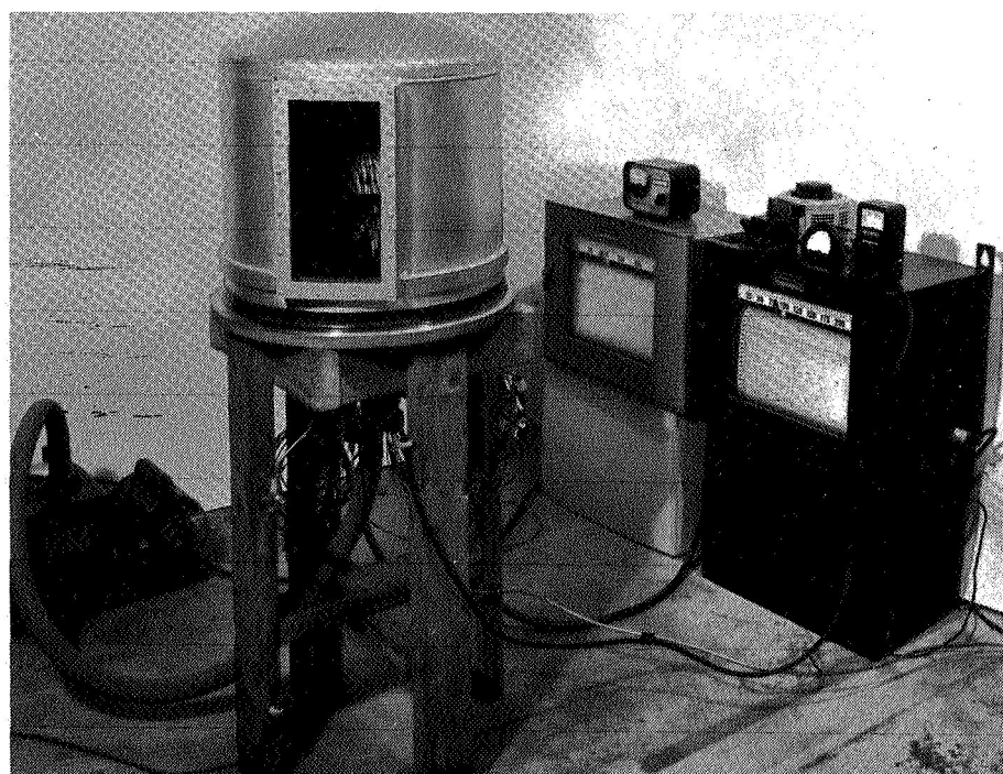
FIGURE V-6 EXPERIMENTAL ARRANGEMENT FOR HEAT TRANSFER STUDY (BELL JAR IN PLACE)
