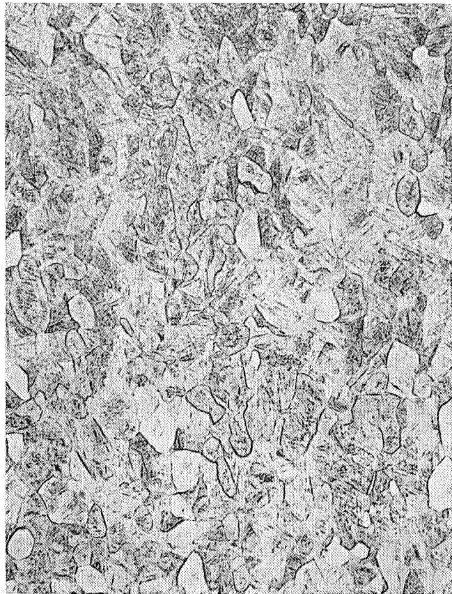
Fig. 42. Microstructure of aft dome, location 7 (500X)
