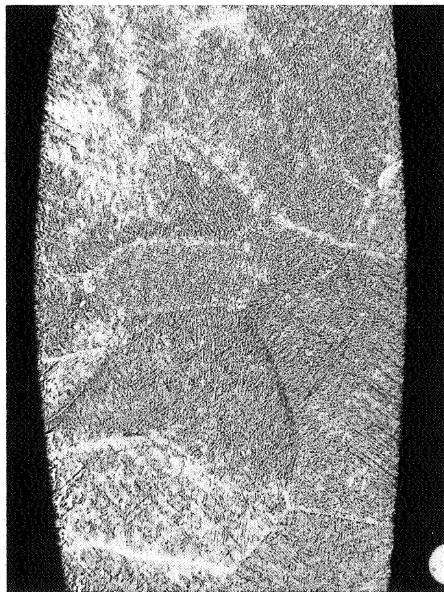
Fig. 36. Microstructure of weld center, location 5 (50X)
