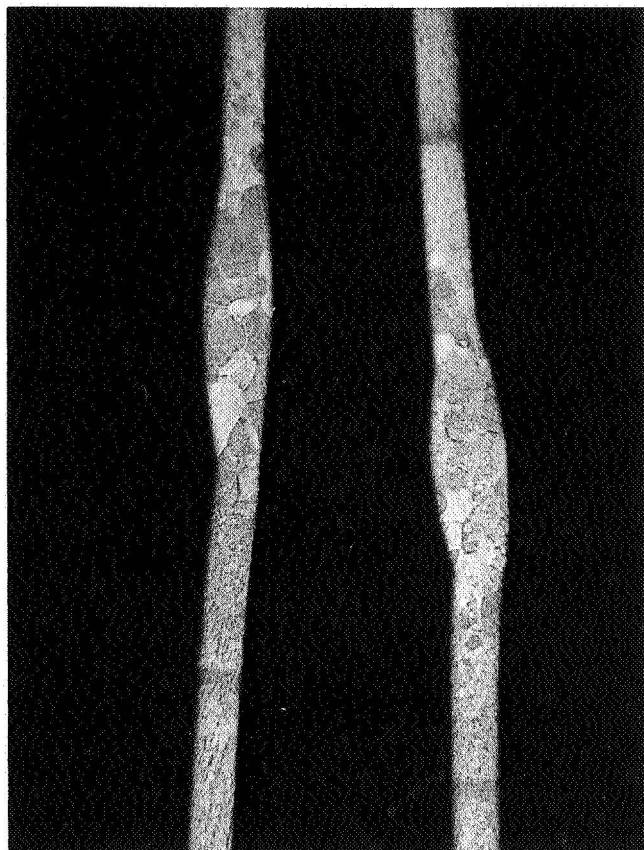
Fig. 35. Macrostructure of welds, location 5 (9X)
