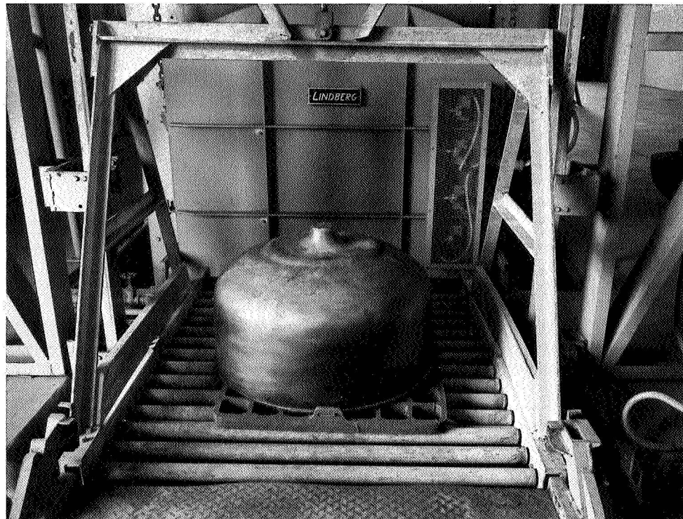
Fig. 12. Forging on quench rack
