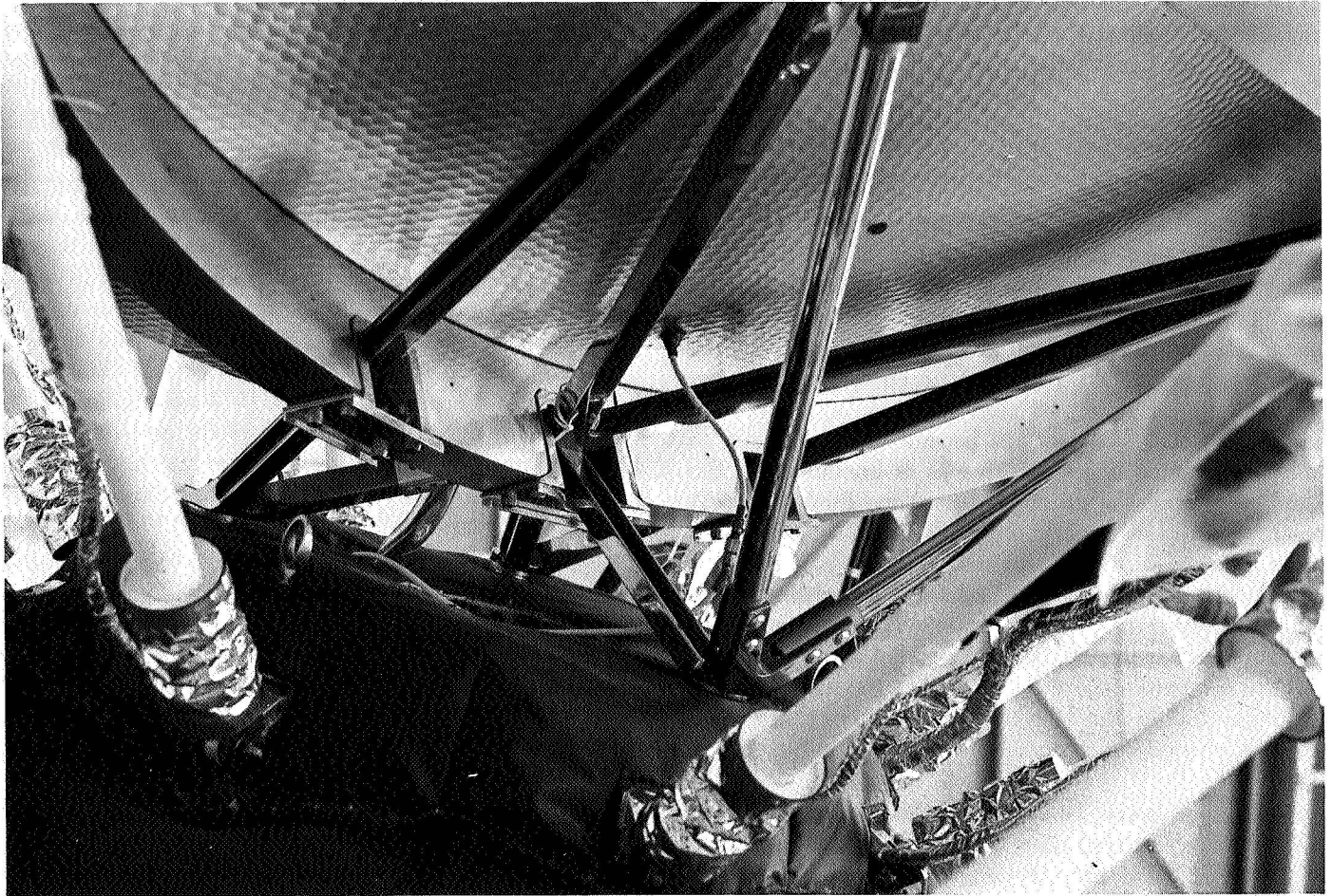
Fig. 5. Antenna support truss
