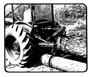
Exclusive automatic grabs\* enable operator to hook and release logs without dismounting from tractor. Note that no cumbersome chains and cables are required.
