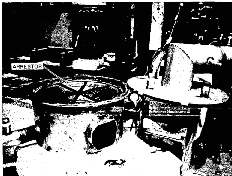
FIGURE 2. Arrestor in Surge Tank.
