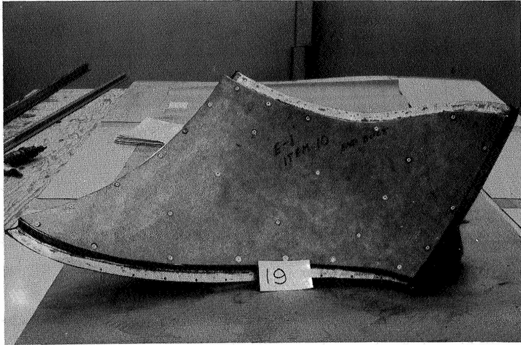
(e) Top cover with 25-rayl fibermetal in place.
