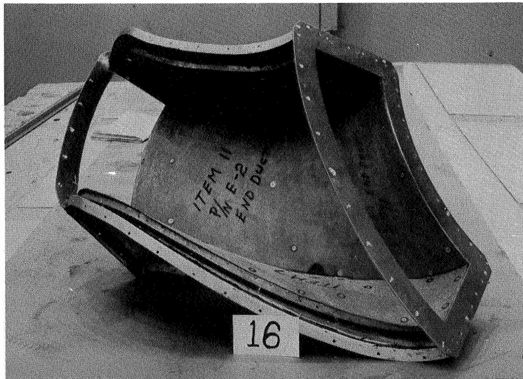
(f) 3/4-front view from duct inlet with 25-rayl fibermetal in place on three walls.
