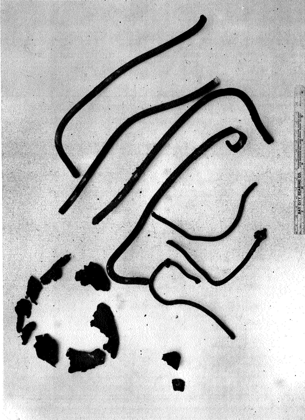
Fig 6 Remains of explosive charge holder with spacer assembly after detonation of 160 grams of explosive while in capsule
