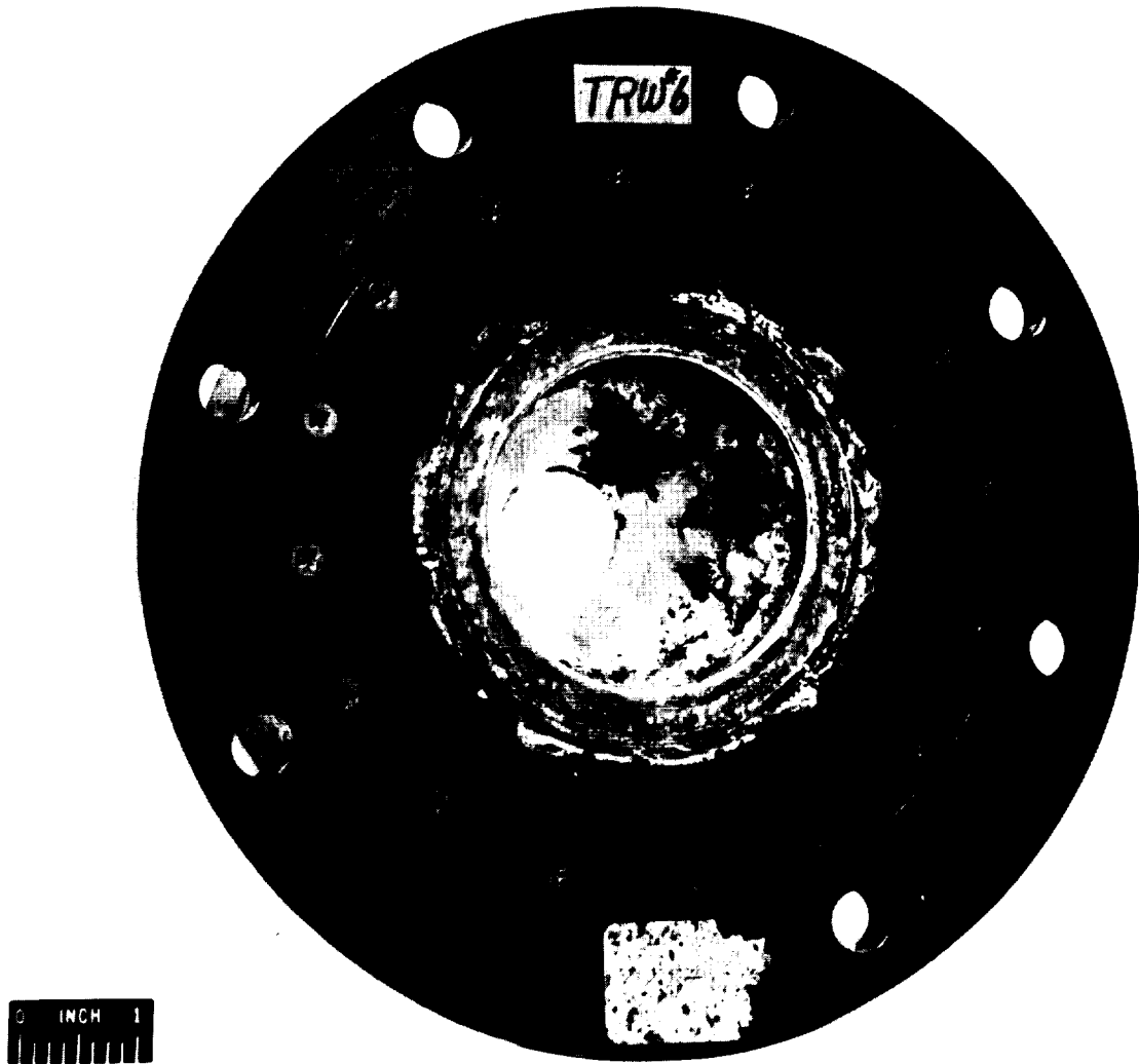
POST TEST VIEW--REINFORCED OXIDE INSERT (II)
