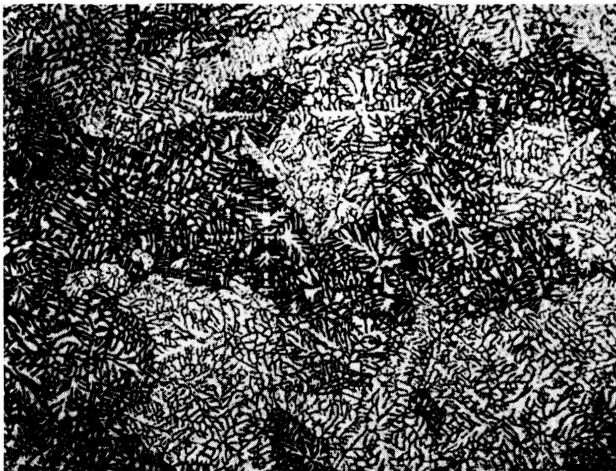
300 amp. 24 i.p.m. 43,600 p.s.i. tensile strength M5651
