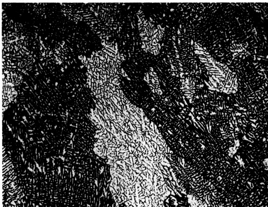
240 amp. 16 i.p.m. 47,600 p.s.i. tensile strength M5650
