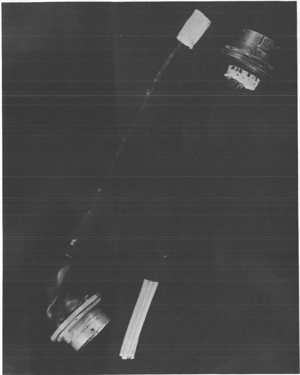
FIGURE 16. Electrical Harness Samples (PT2-96-196, Removable Type Contacts) before ETO-Freon 12. Color Photo (Neg. #32615-67)
