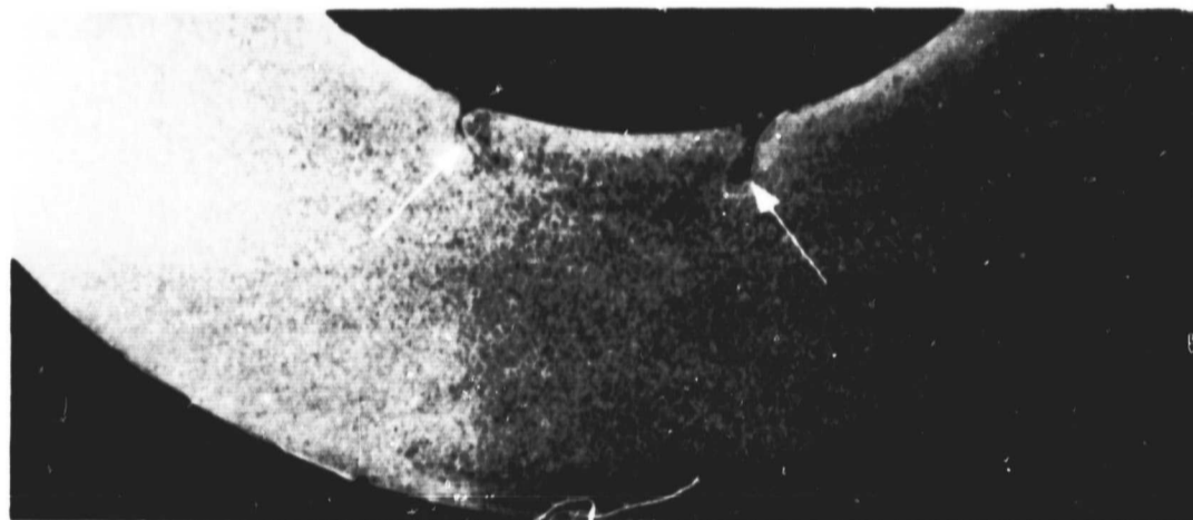
✓ A SURFACE COLD SHUT
