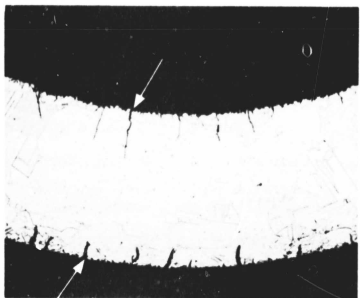
D MICROGRAPH OF CONVOLUTION WITH PARTIAL CRACKING ON SIDES
