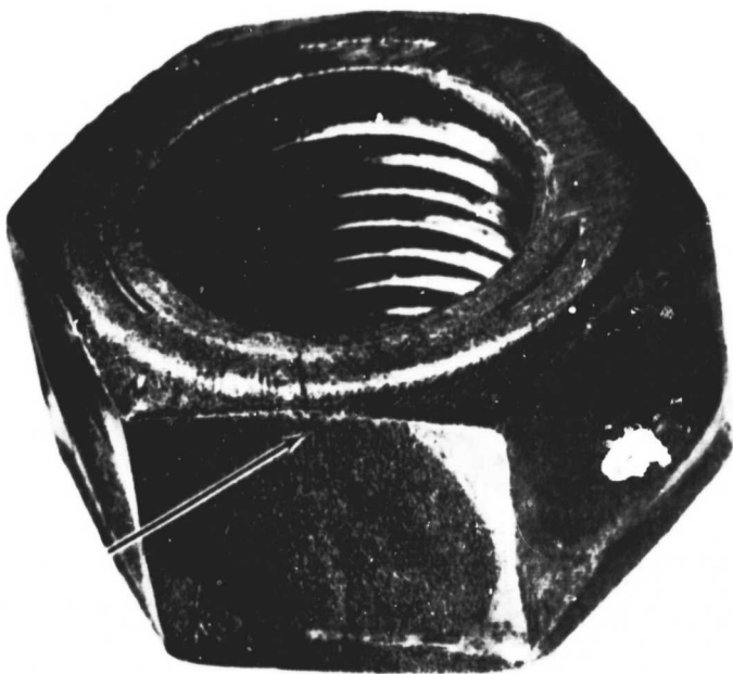
A TYPICAL FORGING LAP
