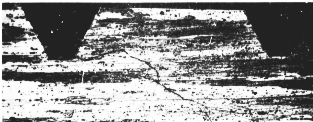
B FAILURE OCCURRING AT ROOT OF THREAD
