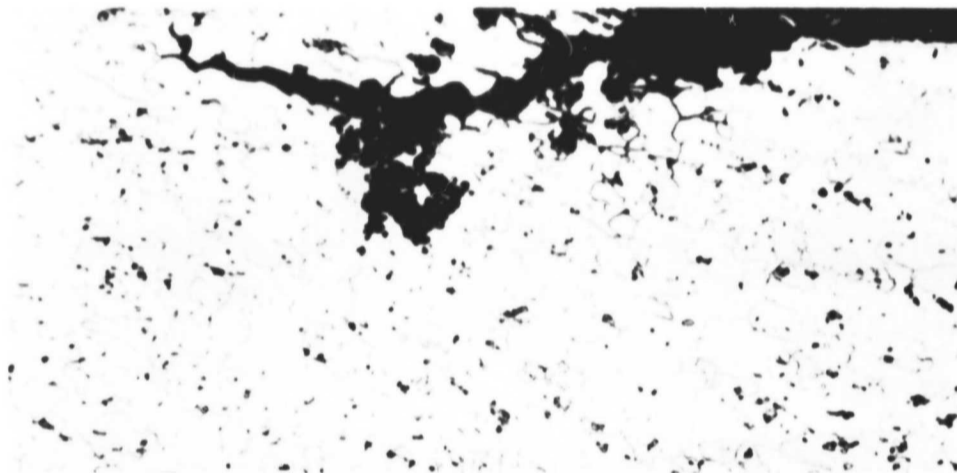
A MICROGRAPH OF INTERGRANULAR CORROSION SHOWING LIFTING OF SURFACE FROM SUBSURFACE CORROSION
