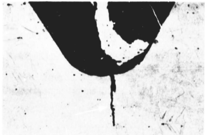
D MICROGRAPH OF (B) SHOWING TRANSGRANULAR CRACK AT THREAD ROOT
