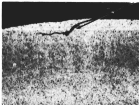
B LAP IN OUTER SURFACE OF TUBING
